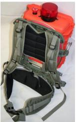
The HT-2000 Battery Backpack Electrofisher is also equipped with two LCD displays. One is the eight-digit seconds counter and the other is a four-digit readout connected directly to the multifunction meter. The multifunction meter can display mean current, peak power, and battery voltage.
