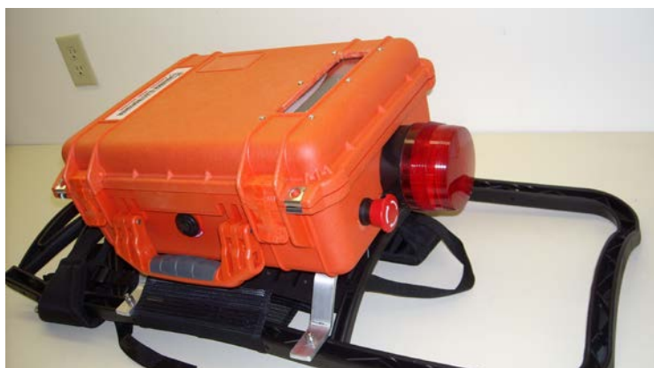
.Red "Power On" Strobe Light .Emergency Off Switch
